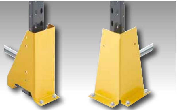
'U' shaped protector gives 3-way protection to the upright
